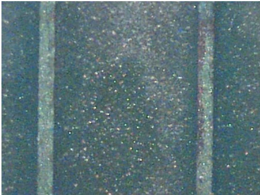
Pattern QFP80 Comb (solder mask discoloration) – Board 4
