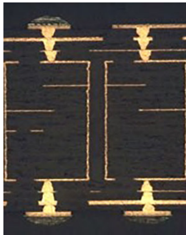
Figure 3: Resin fill—stacked vias.
