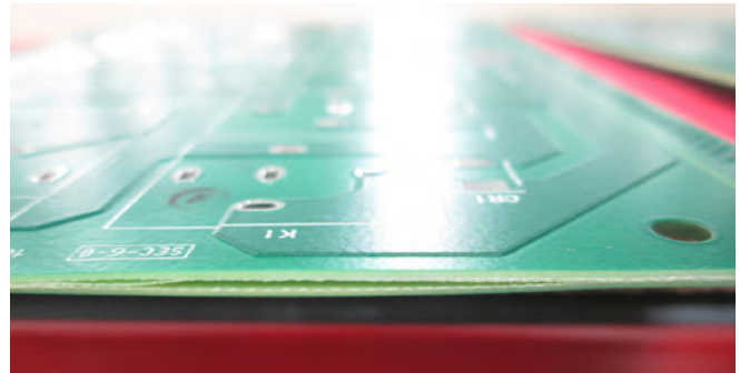
Figure 4: Example of board delamination.
