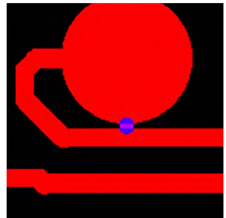
Figure 3: Manufacturing process tolerances can cause a same-net short, potentially affecting circuit behavior.
