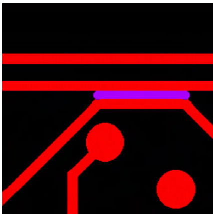
Figure 1: Close spacing over an extended length affects yield and reliability.
