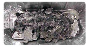
After just one hour in the AKILA unit, dross is converted to usable solder.
