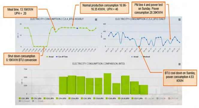
Figure 6: Detailed SMT reflow oven power consumption information.
