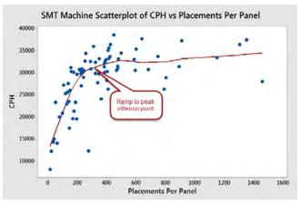
Figure 2: Scatter plot of CPH versus placements per panel from SMT machine product simulations.
