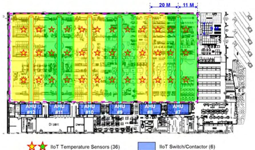
Figure 7: IIoT control vs. line layout (control air conditioning).
