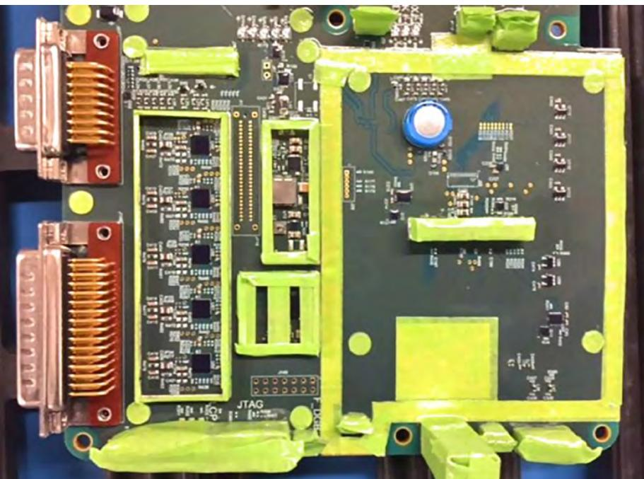
Figure 1: Pre-cut tape shapes for masking.
